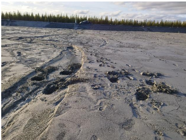
Picture of sample W010_TB_50_A.B.C. and W010_TC_50_A.B.C. Samples was taken inside and outside of tailings flow channel. Samples were taken on depth of 5-6 cm
