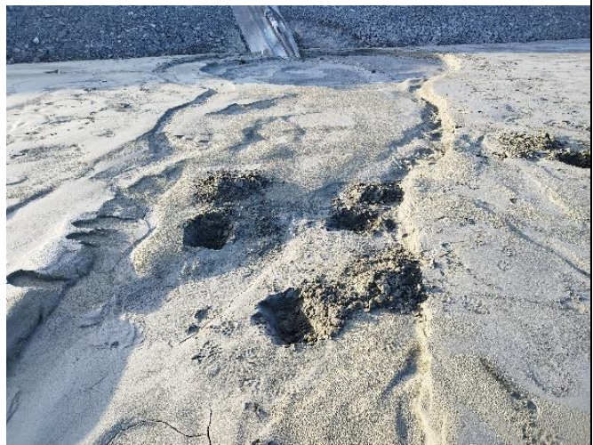
Picture of sample location W010_TC_10_A.B.C. Samples was taken inside of tailings flow channel. Samples were taken on depth of 5-6 cm.
