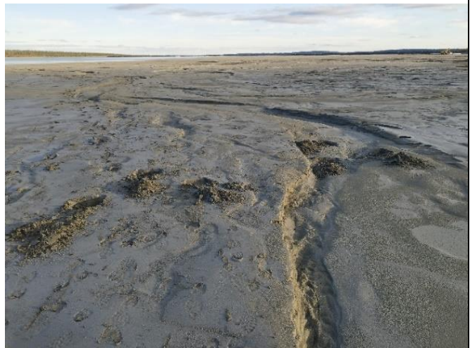
Picture of sample W010_TB_100_A.B.C. and W010_TC_100_A.B.C. Samples was taken inside and outside of tailings flow channel. Samples were taken on depth of 5-6 cm
